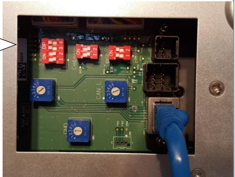
4. Connect a RJ45 patch lead from the CAN on the **blue** Advanced Comm card to the RESU battery.
